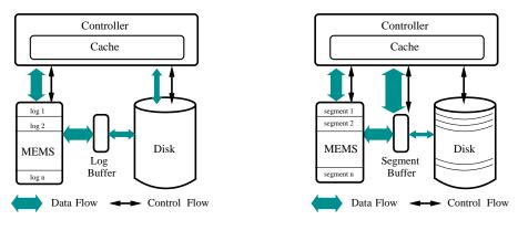
Fig. 6. MEMS Write Buffer.
