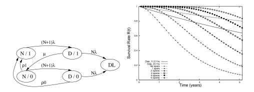
Fig. 2. Markov model for a MEMS storage enclosure. Fig. 3. Survival rate of MEMS storage enclosures without repairs in five years.
