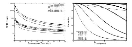
Fig. 4. *MTTF* of MEMS storage enclosures under different maintenance strategies and repair rates.
