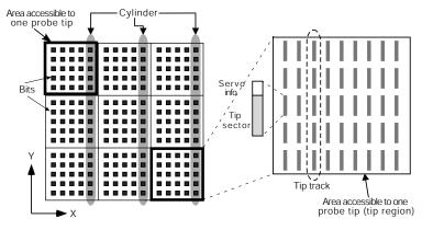
Fig. 1. Data layout on a MEMS device.
