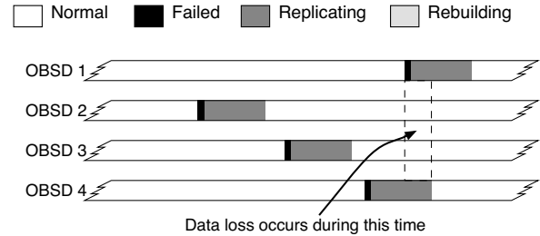
(a) A second OBSD failure within the window of vulnerability from the first causes data loss.
