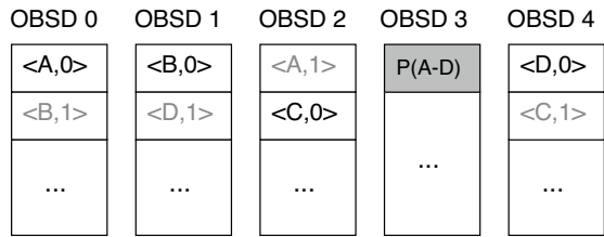
(b) Parity calculated across data on different OBSDs. The second replica from each redundancy set (shown with grayed-out identifiers) can be reclaimed to save space, or can be retained for added reliability.
